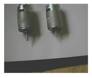
The picture on the left shows two motors, the one on the left modified as described. The one on the right is fitted with two M3 screws which are at the right pitch to allow the motor to be fixed to a Meccano Flat Plate with screws separated by one hole The shaft then sticks through the central hole.
