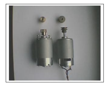
The picture shows, on the right, a motor with a sleeved shaft and fitted with a standard ½" Pulley. The motor on the left is fitted with a 1/8" bore 19 Tooth Pinion the shaft being unmodified. For comparison each motor has a second drive wheel placed in front of it identical to the one on the motor shaft.
